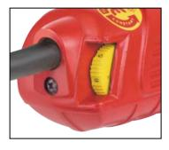
Electronic Speed Regulator adjusts tool speed from 800 to 1800 RPM, and locks in constant speed while tool is in use.
