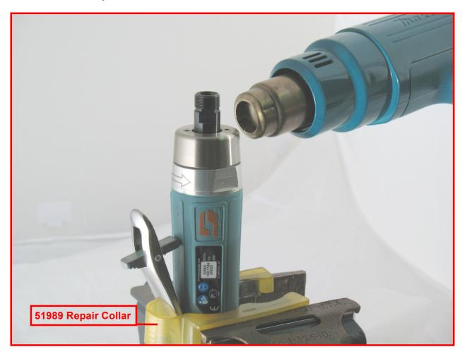
1. Position the **51989** Repair Collar around the motor housing. Fasten the tool in a vise so that the work spindle is pointing up. Use a HEAT GUN to warm the **51947** Housing Cover and soften the thread adhesive.
