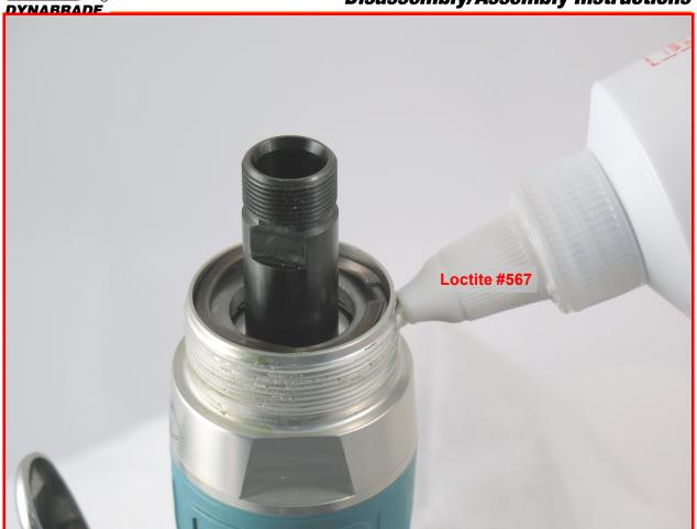
Apply a small amount of Loctite #567 to housing thread.
