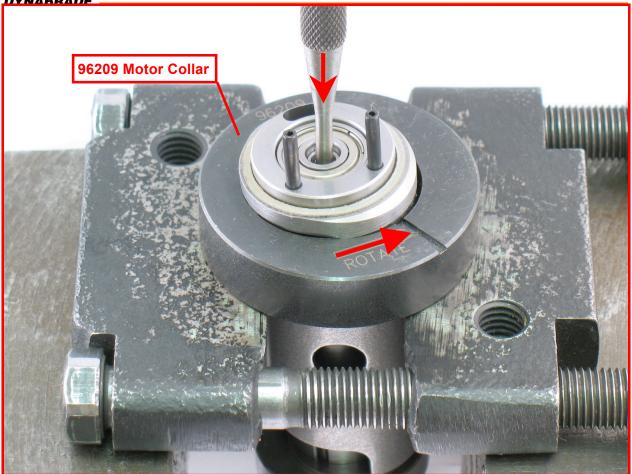
4. Fasten the 96209 Motor Collar around the cylinder, near the rear bearing plate.
