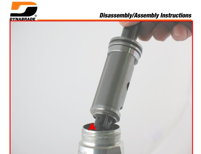
**2.** Pull-up on the work spindle to remove the motor with the **96498** Wave Spring, and the **53620** Motor Adapter from the housing.
