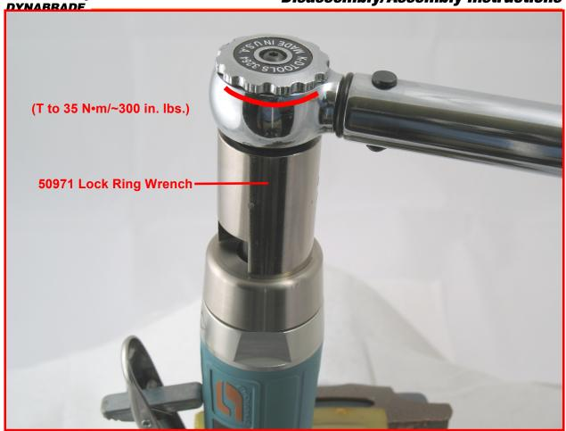
Use the 50971 Lock Ring Wrench and torque wrench to install 51947 Housing Cover. (T to 35 N•m/~300 in. lbs.)
