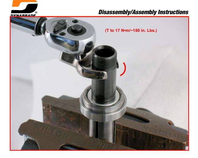
Use a 14 mm crowfoot and torque wrench to fasten the 50011 Collet Body onto the rotor.
