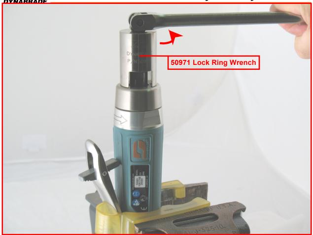
Use the 50971 Lock Ring Wrench or an adjustable pin wrench to remove the 51947 Housing Cover. Turn counterclockwise.
