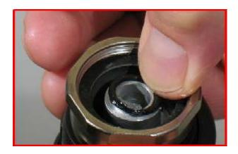
**4.** Apply a small amount of clean grease to the **95523** O-Ring and install it onto the throttle body.
