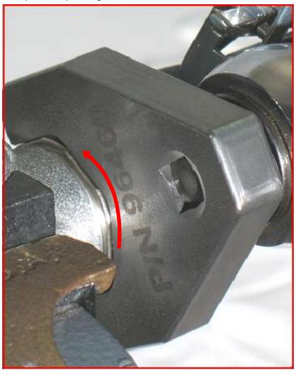
2. Pull the 01558 Collar back onto the throttle body. Use the 96460 Wrench to loosen the throttle body from the 7°housing. Left Hand Thread Turn clockwise.
