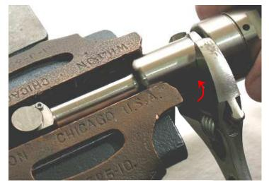
Use a 5/8" or 16 mm hex key to remove the 54540 Retaining Nut. LEFT HAND THREAD Turn clockwise.
