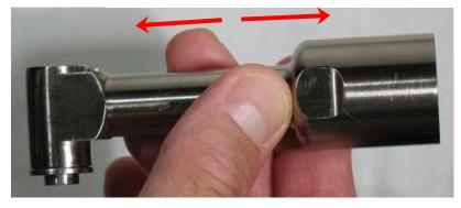
If there is movement, use the **54536** Shim Pack and add shims as required. **Notice:** Shim pack contains .002" (0.05 mm) and .005" (~0.13 mm) thick shims.
