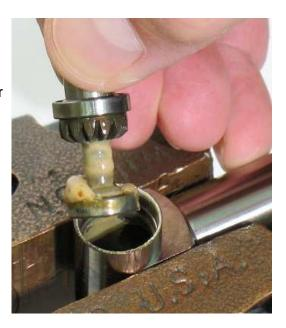
**Angle Head Disassembly Complete.**
