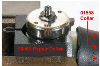
3. Fasten the 01578 or 94523 Inlet Adapter in a vise with aluminum or bronze jaws so that the throttle body is pointing up.
