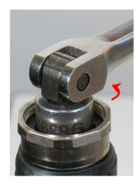
**4.** To disassemble the muffler and valve components, refer to, and follow the exploded view instructions found in the parts page or tool manual.
