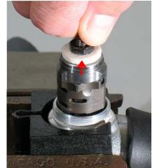
**4.** Remove the motor from the housing.
