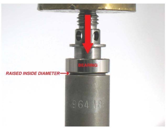
**3.** Use *"RAISED INSIDE DIAMETER*" of **96418** Bearing Press Tool, and **96232** Arbor Press to install **51651** or **51686** Bearing onto drive shaft.
