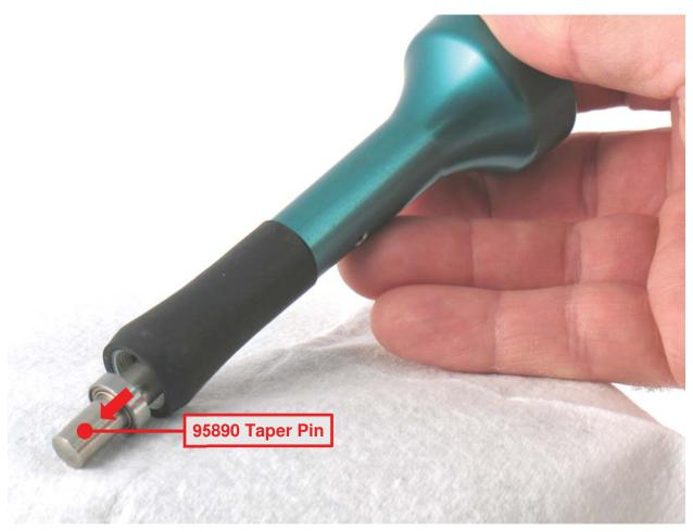
9. Use 95890 Taper Pin, or a 9 mm (~.354") diameter rod, as a ram to remove 51544 or 51685 Bearing from housing.
