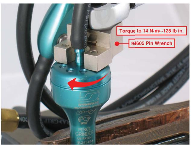
**15.** Insert **51694** Pin through cross-hole in housing and drive shaft and fasten in vise.
